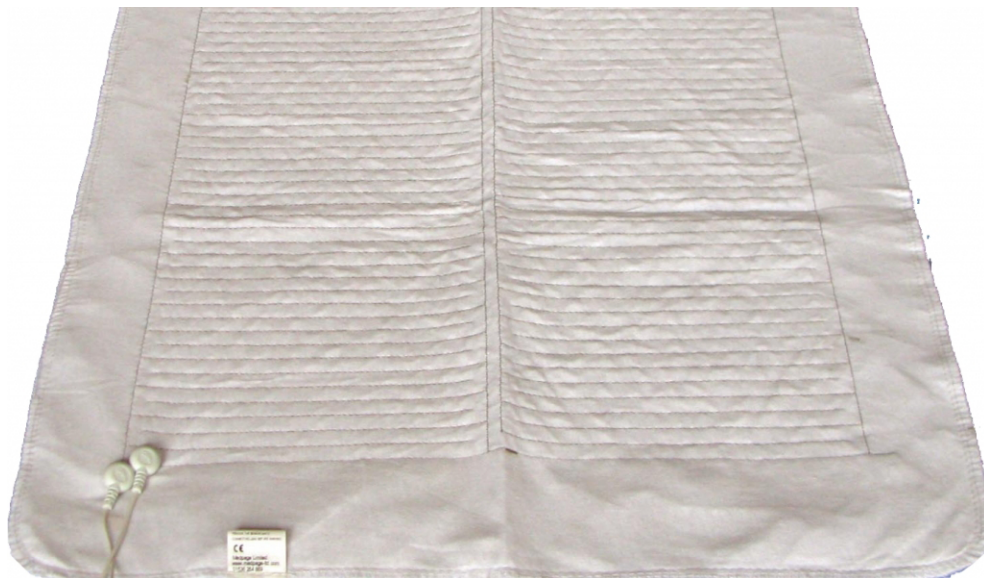
34 Enuresis Sensor that can be connected to Telehealth system.
